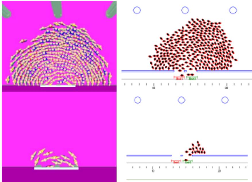
**Fig. 10.** Difference in evacuee distribution between exits in *FDS+Evac* (left) and *Simulex* (right) on two different time steps. In *FDS+Evac* the evacuees choose the fastest way out, in *Simulex* the evacuees take the shortest way out.
