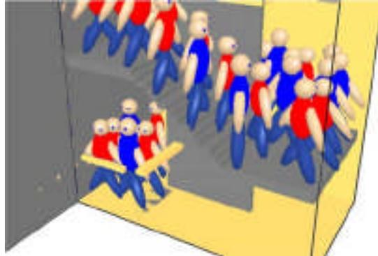
**Fig. 11.** When two different rows of evacuees had to intercalate, the door became obstructed several times for several seconds in FDS+Evac.
