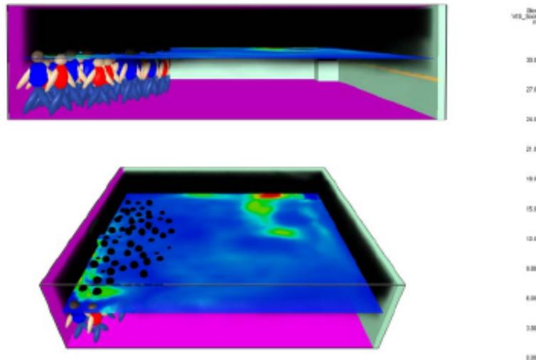
**Fig. 7.** This figure shows the evacuees in the room obstructing the door. Also the smoke layer is visible and the *visibility* is shown on 1.50 meter height. *Dark blue* means, *no visibility* at all (0 meter) *red* means a visibility of 30 meter.
