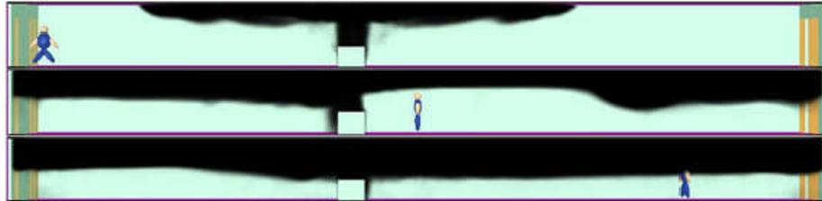
**Fig. 6.** Graphic view of FDS+Evac after 0, 15 and 30 seconds, with lot of smoke production simulated.
